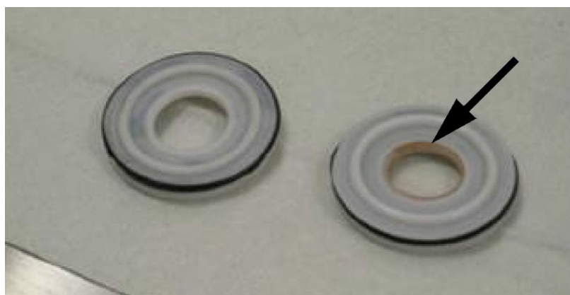
Figure 5.E-7 Reddish-brown deposits in a PTFE seal. The rouge particles transported in the WFI have been deposited on the seal. (Source: Henkel Beiz- und Elektropolier technik GmbH & Co.KG, 19306 Neustadt-Glewe, Germany)
