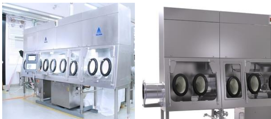
Figure 4.I-12 Process isolator for the blister-packaging of tablets (courtesy of SKAN AG)
