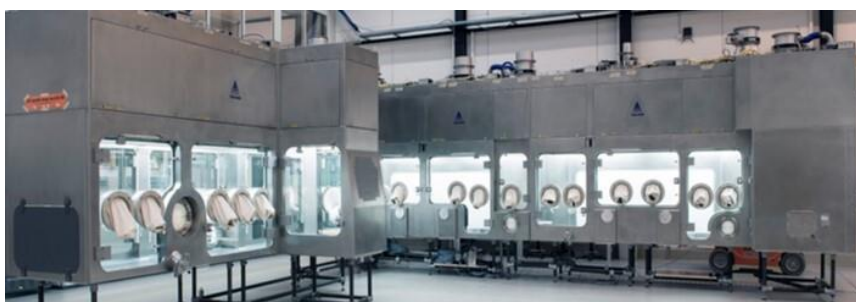
Figure 4.I-15 Completed isolator built according to mock-up study results (courtesy of SKAN AG)
