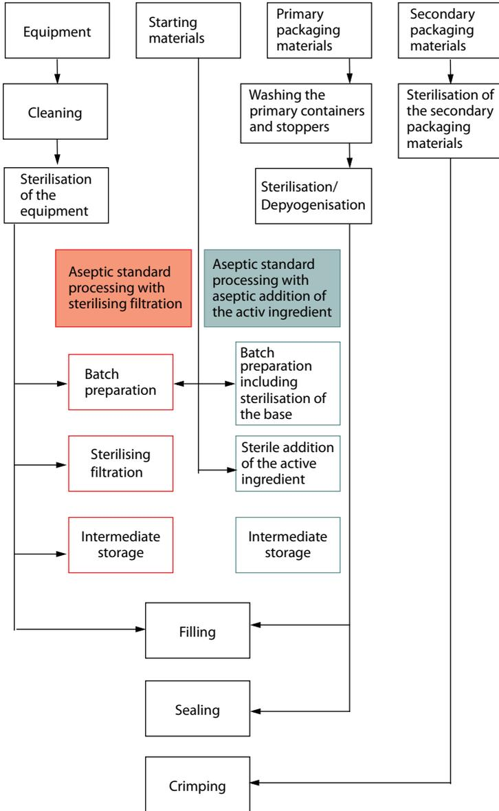
Figure 1 Schematic diagram of aseptic processing by means of sterile filtration and the addition of sterile active ingredients
